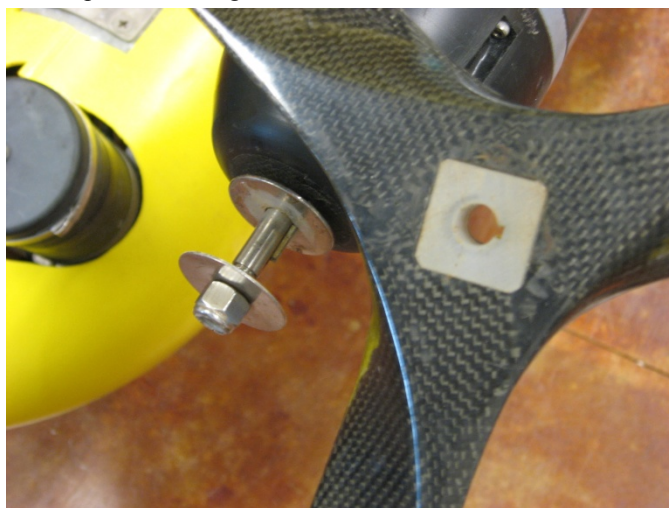
Figure 5. Redesigned propeller hub and keyed shaft.
