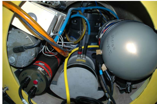
Fig. 2 Tethys Mass Spectrometer installed in Eagle Ray AUV. Image shows from left to right Syntactic Foam, Battery Housing for Acoustic Modem, External Battery Pack for Tethys, EM2000 Multibeam Receiver, and the Tethys Mass Spectrometer.
