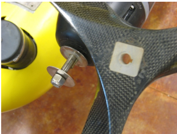
Figure 8. Redesigned propeller hub and keyed shaft.
